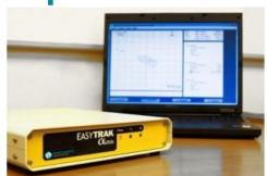
Applied Acoustics unveiled their USBL tracking system at Oceanology International. Called the Easytrak Alpha, it is the introductory and most compact of their range of subsea tracking systems. Ideally suited for small vehicle operations or basic diver tracking, Alpha is a condensed and cost-effective system for monitoring close range subsea targets.
