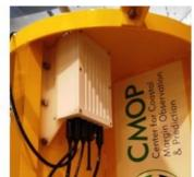
The University of Washington (Seattle, USA) recently deployed an oceanographic observing buoy featuring Soundnine Inc.'s DANTE System. The DANTE controller collects data from a suite of meteorological and oceanographic instruments. Two sensors are 60 feet underwater and use S9's Ulti-modem inductive modem to communicate with the controller on the surface.
