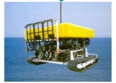
DeepOcean, UK, took delivery of two TSS 440 and two TSS 350 pipe/cable tracking systems at the start of the summer season and has been using them regularly since then. The systems are occupying an essential role in DeepOcean's equipment inventory. The Teledyne TSS systems can be used for cable and pipe tracking which is essential for many of these tasks, and DeepOcean is now making good use of their capabilities.
