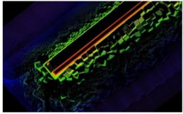
NORBIT Subsea's Release 10.0 is the updated firmware/software package increasing the performance of the <u>WBMS family of systems</u>. It realises high-resolution sidescan-snippets (which take full benefit of the cylindrical array and the 80kHz FM bandwidth), roll stabilisation over 160° swath (Applanix interfaced), flexible water column display / output and enhancements to the intuitive user interface.
