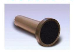
The single-beam LinkQuest FlowScout 600 acoustic flow meter is based on innovative acoustic Doppler technology and is capable of reaching up to 110 metres in range with an accuracy of up to 0.5% +/- 2.0 mm/s. The operating frequency of the FlowScout 600 system is 600kHz. The standard depth rating of the system is 100m.
