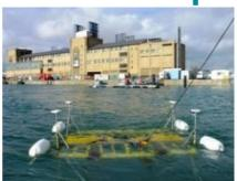
The GeoChirp 3D from GeoAcoustics Ltd provides the shallow-survey market with a new tool to image sub-surface structures and buried objects. The GeoChirp 3D provides a three-dimensional image of the sub-seabed with typical penetration of 10 – 30m and decimetric horizontal and vertical resolution, with the results presented as a high resolution 3D seismic volume.
