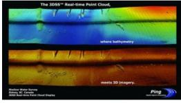
Geometius, based in The Netherlands, has become European distributor of the 3DSS-DX-450, developed and manufactured by Ping DSP based in Victoria (Canada). The 3DSS-DX-450 is a 3D sidescan sonar that produces swath bathymetry and 3D sidescan imagery based upon the unique CAATI technology. This patented technology is able to resolve multiple concurrent acoustic arrivals, separating backscatter from the seabed, sea surface, water column and multipath arrivals.
