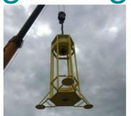
UK-based Ocean Scientific International Ltd (OSIL) has introduced a lightweight version of its Vibrocorer. The lightweight vibrocorer is roughly half the weight of the high-power version, but retains sufficient structural strength and vibration force (30kN) to drive the barrel up to 6m into densely compacted sediments in up to 250m water depth, courtesy of the vibrating motor contained within the sealed pressure housing.
