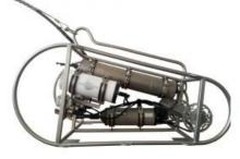
The Observer III Mariscope proposes a solution for scientists that need an underwater MPV. The unit is equipped with 2 HD cameras and 4 HD high output LED lights, apart from batteries and control electronics, facilitating to have one camera looking forward and the other one looking backward. The Observer III can also be equipped with standard Oceanographic sensors like CTDs, CO2, Methane sensors, tracking systems and others.
