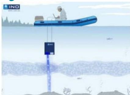
Canadian research institute INO has developed a submarine Lidar to measure the reflectance of the seafloor and water column. The system is used to determine the reflectance of the sea bottom so that the composition can be correlated with relative intensity data from aerial surveys. INO's Lidar system helps to calibrate the results of airborne bathymetric surveys, increasing their accuracy and enhancing understanding of the results.
