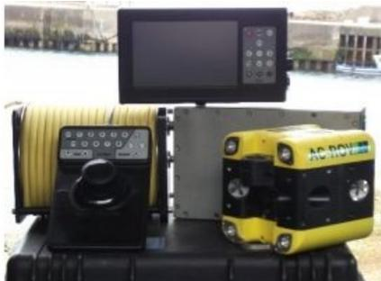
McPherson Ltd, one of the biggest whisky road hauliers in Scotland, have purchased an AC-ROV 100 to examine the internal welds, baffles and valves of their tankers to meet the UK period inspection requirements.
