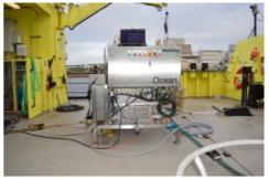
MacArtney Benelux has supplied a CORMAC M4C winch to Belgian dotOcean, specialised in sediment and soil characterisation systems and instrumentation. This is a customised version of the MacArtney CORMAC M modular winch series intended for use together with the dotOcean DensX sediment density profiler. DensX is an in-situ, direct measurement mud density method using safe X-ray technology and an automated winch.
