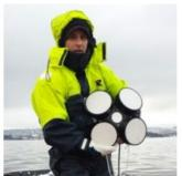
The mid-range profiler Nortek Signature 250 is now in production. It has an optional centre beam for the patented SUV wave measurement mode, which means it can be deployed on subsurface buoys at depths up to 150 metres. The Signature family now includes instruments covering ranges from <1m to >1,000m (frequencies of 1000, 500, 250 and 55kHz). Hence, the Signature series now covers most needs and requirements in terms of range and application.
