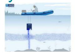
Canadian research institute INO has developed a submarine Lidar to measure the reflectance of the seafloor and water column. The system is used to determine the reflectance of the sea bottom so that the composition can be correlated with relative intensity data from aerial surveys. INO's Lidar system helps to calibrate the results of airborne bathymetric surveys, increasing their accuracy and enhancing understanding of the results.
