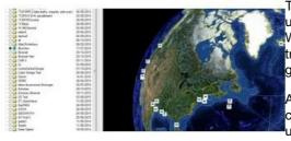
Teledyne PDS 4.1 software features Visual Project Management and Setup. It includes a user interface which provides a visual presentation of the survey tracks on the world globe. When zoomed in on, it will appear as a flat plane to be viewed in detail showing the GPS tracks data and the extent of the projects. Project information is available on the world globe or in the projects list.
