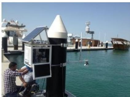
OceanWise is working with Seatronics to complete a three-year project to design, install and deliver a fully operational network of 34 water level and temperature monitoring stations for Bayanat LLC in the United Arab Emirates (UAE). The stations are positioned at strategic locations within UAE from the Western Region to the border with Oman, covering a distance of over 400km.
