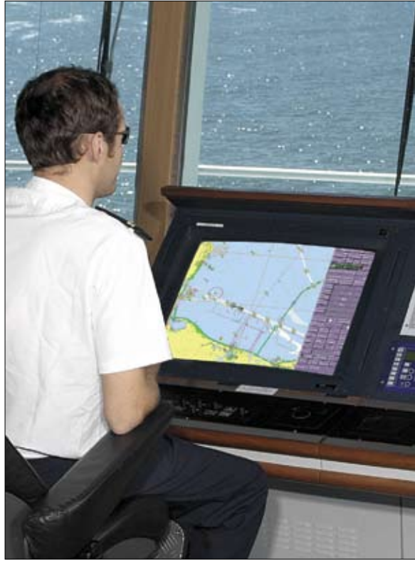
Figure 1.2: Watch Officer navigating with an electronic chart. Source: Sperry Marine (Northrop Grummon).
