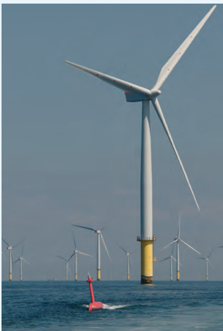
▲ Figure 1: DriX conducting a bathymetric survey on Gwynt y Môr offshore wind farm off the coast of Wales.
