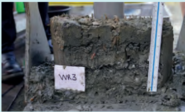
▲ Side view of a box core showing the top few decimetres of seabed sediment. (Image courtesy: TNO)
