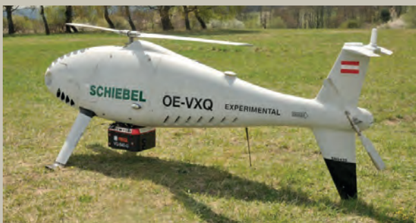
▲ The RIEGL VQ-840-G topobathymetric Lidar sensor mounted on the Schiebel Camcopter S-100 UAS. (Image courtesy: RIEGL)
