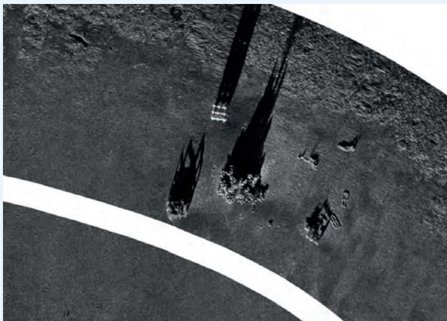
▲ Figure 1: Very high frequency EdgeTech 4205 sidescan sonar (850kHz), acquired by FlipiX over structures on the seabed.
