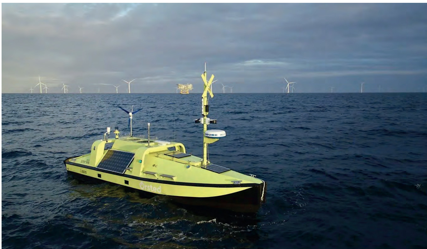
▲ The Hugin USV is anchored at Ørsted's Anholt wind farm, ready to be deployed for offshore metocean measurement campaigns in the wind farm industry. This stands as a good example of the ever-increasing role of autonomous survey methods in hydrography. (Image courtesy: Ørsted)
