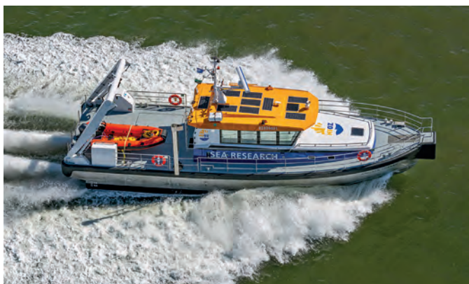
▲ The RV Adriaen Coenen: shallow draft of 85cm, seating for two crew and 12 passengers – ideal for Wadden Sea tidal flats, able to rest on sandbanks during high tide. (Image courtesy: NIOZ)
