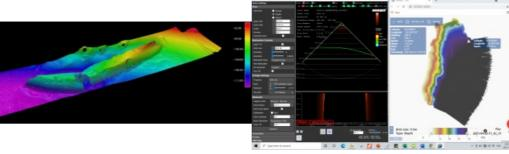
The key objective was to make a rapid and accurate determination of the source of the diesel and oil that had appeared on the ocean's surface. The company carried out hydrographic survey work using a Norbit Winghead i77h multibeam echosounder (MBES) system. The team deployed the device both from the surface, mounted onto a
