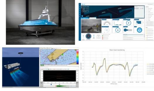
Aquatic Drones, based in the Netherlands, recently introduced the Phoenix 5 Autonomous Surface Vessel (ASV). The unit, with a length of five metres, provides a stable platform for a range of survey and inspection operations. It can be deployed for bathymetric surveys, sub-bottom profiling, inspection of civil engineering structures, safety and security surveillance, water quality monitoring and other applications. Phoenix 5 is designed for operations on inland waterways, in ports and nearshore.
