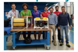
Lighthouse has delivered an <u>AGEOTEC ROV Sirio</u> to Tripodij Doo, a Croatian company based in Dugopolje (Split, Croatia). This ROV Sirio, configured according to specific customer requirements, has been equipped with a Tritech USBL Micronav 100 and a 1 function manipulator with a cutting cable unit. The AGEOTEC ROV Sirio has been successfully tested in the swimming pool, where the factory acceptance test was positively conducted.
