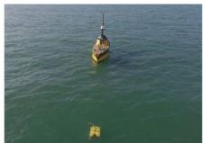
L3 Technologies has launched an Autonomous Surface Vessel (ASV) deploying, operating and recovering a Remotely Operated Vehicle (ROV). In an industry first, the C-Worker 7 ASV deployed an inspection-class ROV for vertical and horizontal subsea inspection. The proof of concept demonstration took place over two weeks in Cawsand Bay, Plymouth, UK. The system will be running demonstrations at Ocean Business in Southampton, UK, 9-11 April 2019.
