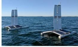
Norwegian offshore wind developer Equinor and US-based start-up Autonomous Marine Systems (AMS) have launched a 16 ft autonomous sailing platform to cut the cost of gathering data needed for developing offshore wind projects. The wind and solar-powered Datamaran vessel, developed by AMS, carries a LiDAR device to collect data on wind and weather conditions at remote offshore wind lease areas.
