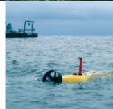
For those unfamiliar with AUVs, it is a robotic platform that operates underwater and is typically powered by batteries and it has no physical link to the surface. The missions undertaken by AUVs are typically pre-programmed and the AUV is capable of carrying multiple sensors which gather data of the environment. For hydrographic applications, the AUV has demonstrated that is capable of acquiring
