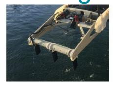
Innovatum have successfully tested Smartrak, a fully autonomous passive magnetic tracking system of a submarine cable by Autonomous Underwater Vehicles (AUV). An AUV Data Protocol has also been developed providing a standard communication format between Smartrak and the AUV.
