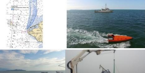
TerraSond, a hydrographic services company based in Palmer, Alaska (USA), utilised an unmanned Autonomous Surface Vessel (ASV) to assist with the acquisition of survey data in July of 2015 in the northern Bering Strait region of Alaska. The 12' ASV, a military target drone converted into a hydrographic vessel, worked in conjunction with a larger survey vessel and acquired the first data from an unmanned vessel to be used to update a US nautical chart.
