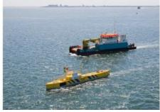
electricity from the tides, where tidal turbines are installed on the seabed, require high-end offshore installation vessels and do not allow for easy access for maintenance. The BlueTEC floating tidal energy platform has a different approach. It is a permanently moored platform which generates renewable electricity from tidal currents by holding a tidal turbine underneath. The BlueTEC Texel is the first prototype and serves as a demonstration platform and is being used for R&D testing purposes.
