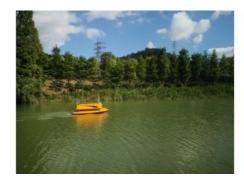
In order to detect any sudden outbreak of water pollution in the city's main river, the government department of Zhengjia, a coastal city in China, introduced an unmanned surface vehicle to its water monitoring routine to detect and restrain all illegal sewage discharge from companies alongside the riverbank.
