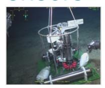
Both in the coastal area and several thousand metres deep, COSTOF2 can power and control submarine observation station sensors and retrieve their data in real time. This tool was developed by Ifremer and transferred to the RTsys company, which is now industrialising it.
