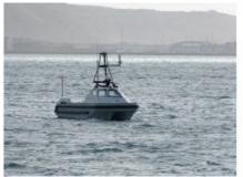
Successful sea trials have been conducted to demonstrate the integration of the ATLAS ELEKTRONIK UK (AEUK) ARCIMS unmanned surface vehicle (USV) with SeeByte's Neptune autonomy software. In challenging conditions with winds gusting up to 45mph, the ARCIMS USV was controlled by SeeByte's Neptune system in a number of autonomous missions in Portland
