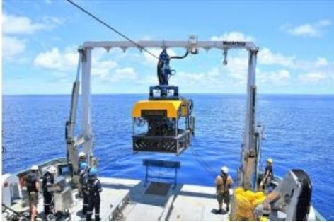
The MacArtney MERMAC D docking head onboard the RV 'Falkor' for the Schmidt Ocean Institute ROV 'SuBastian' has been designed featuring one single suspension point. In consequence, its design and functionality ensure safe launch and recovery of the ROV system as well as stability and steadiness in heavy seas without unexpected movement of the systems.
