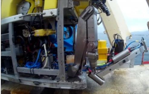
In December 2016, DOF Subsea (DOF) conducted a demonstration of dynamic underwater laser scanning as a replacement for traditional metrology techniques at The Underwater Centre in Fort William, Scotland. The demo showcased 2G Robotics' and Sonardyne's complete dynamic survey solution.
