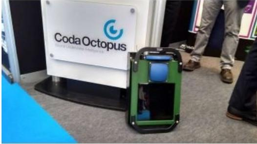
At Coda Octopus' stand Q9 at Ocean Business 2017 visitors find an addition to the real-time 3D sonar range, the Echoscope XD. The Echoscope XD sees a wide-angle 90° x 44° 240kHz option added to the Echoscope. This new variant of sonar has multiple projectors and allows a wider field of view.
