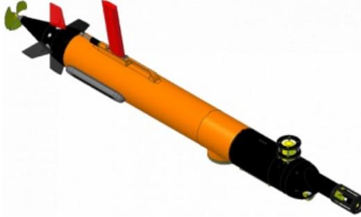
Explorer Doppler Velocity Logs (DVLs). They have been successfully integrated on OceanScan-MST's™ light autonomous underwater vehicle system (LAUV), which is an affordable and innovative one-man portable AUV that can be easily launched, operated and recovered with minimal setup.
