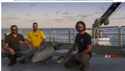
The unmanned aircraft with a wingspan of 3.6 metres will take off from research vessel 'Falkor' to scan the sea surface with cameras and highly sensitive thermal and optical measuring instruments.
