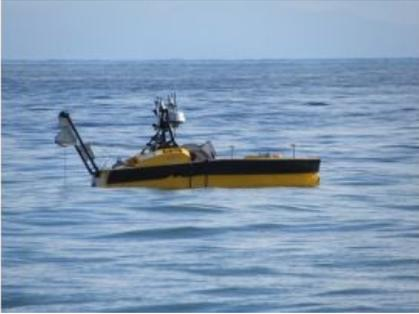
ASV Global and TerraSond have completed their first ever seabed cable route survey supported by an unmanned surface vehicle (USV). The survey route included various water depths and strong currents, while facing difficult wind and sea conditions in the Bering Sea offshore Alaska. The project was mobilised immediately following a 9,000km nautical charting survey by TerraSond, of which 4,750km (53%) were executed by an ASV Global C-Worker 5 autonomous surface vehicle (ASV).
