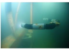
Eelume AS has released live video footage of its underwater intervention vehicles. With the support of Kongsberg Maritime as a development partner, the Eelume robot has presented itself as a snake-like vehicle designed to live permanently underwater and carry out underwater intervention tasks that would normally require the mobilisation of expensive surface vehicles for divers or
