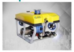
H300-V is a new ROV launched by ECA Group at the occasion of Underwater Intervention 2017. It is dedicated to observation and inspection missions. The H300-V ROV has been developed to meet the demanding markets using observation-class ROVs in harsh environments. Powerful while portable and compact, H300-V is a new vehicle designed and tested upon a full range of requests coming from worldwide ROV users.
