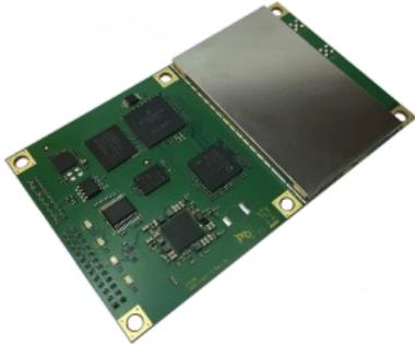
Today, Hemisphere GNSS has announced the Eclipse P328 in a line of low-power, high-precision, positioning OEM boards. The multi-frequency, multi-GNSS P328 is an all-signals receiver board that includes Hemisphere's new hardware platform and integrates Atlas GNSS Global Corrections.
