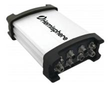
Hemisphere GNSS has introduced the all-new Vector V1000 GNSS receiver, which provides high-accuracy heading, position, pitch, roll and heave data. The V1000 supports multi-frequency GPS, GLONASS, BeiDou, Galileo, QZSS and IRNSS (with future firmware upgrade and activation) for simultaneous satellite tracking. The V1000 is powered by Hemisphere's innovative and industry-leading Athena RTK engine and is Atlas L-band capable.
