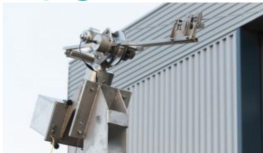
On behalf of its client Boskalis, Dutch subsea technology company Seatools has completed the upgrade of a HighWire survey grade taut wire system. The upgraded position reference system will be deployed to determine the position of a subsea cable plough during a subsea cable installation project executed by Boskalis.
