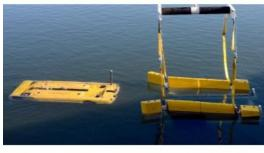
The Modus hybrid is one of the first autonomous underwater vehicles (AUVs) to feature the capabilities and characteristics of a remotely operated vehicle (ROV). Modus Seabed Intervention has completed system integration and trialling of one of the subsea industries first commercially available hybrid unmanned underwater vehicles, thus driving performance, quality and cost-effective delivery of survey and inspection projects in the offshore, defence and oceanographic sectors.
