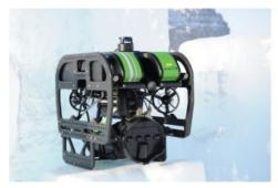
The Kongsberg M3 Sonar system can be mounted on the <u>Teledyne Seabotix vLBV Observation Class ROV</u>. The M3 Sonar is a 2D multibeam echosounder system with sophisticated imaging and profiling capabilities. It provides high-resolution and easy-to-interpret images by combining the rapid refresh rate of conventional multibeam sonar with image quality comparable to a singlebeam sonar.
