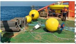
MSI has been awarded a major metocean contract and successfully deployed a large metocean mooring array offshore Tanzania for Shell (formerly BG). With water depths ranging from 53m to 2,620m, the array comprises 2 AXYS Technologies Watchmate metocean buoys as well as 12 subsea moorings, measuring waves, currents and water quality parameters. The project is expected to last 12 months and the data will be used as input for engineering design of surface and subsurface structures.
