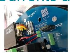
Ocean Scientific International Ltd has added a low-cost, low-power satellite modem to its range of telemetry equipment. The system will publish data (including traditionally high cost/volume currents and waves) from any location globally using the Iridium satellite network. Monthly line rental costs are minimal and data costs are kept low (as little as GBP0.04 per message) by using SBD messaging with big bundle deals available for multiple or long-term deployments.
