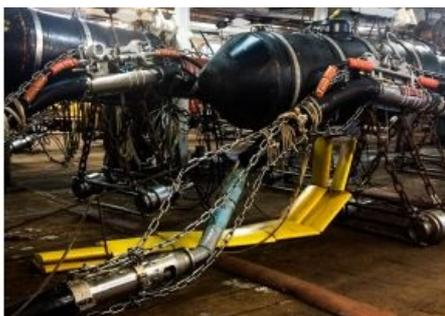
MacArtney & ION have developed a SailWing actuator and control system designed to ensure the correct positioning and stability of seismic survey source arrays. The product has been launched to gather data for enhanced exploration and production of oil and gas.
