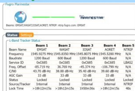
Figure 1: Marinestar transmits corrections over six geostationary L-band beams and internet.
