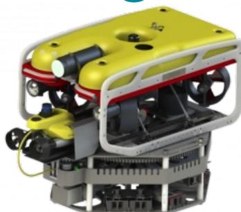
Saab Seeye customer Stinger Technology has developed an idea to penetrate the labyrinth inside offshore production tanks in search of environmental contaminants prior to decommissioning. The company has managed to squeeze an underwater robotic systems configuration loaded with sampling technology through a 150cm-square hatch to search a tank's internal maze of baffles and navigate along 25.5cm-diameter pipe runs of curves and bends.
