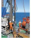
Geotechnical investigations for offshore constructions require continuous technical innovation in order to meet market demands. This is also relevant to the growing offshore wind energy industry, which is itself on a path of constant innovation. The daily costs of offshore operations are high, meaning that honouring a contract satisfactorily and on time is important. To achieve this,
